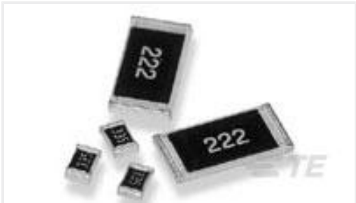
TE Part #2-2176186-7 CRGH1206 1% 18K 0.5W
