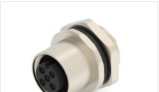
TE Part #T4133012041-000 M12,FRONT MOUNT,FEMALE,A,4P, SOLDER WIRE
