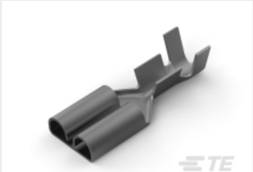
TE Part #179461-5 250 FASTIN FASTON,REC.,20-14 AWG, TPBR
