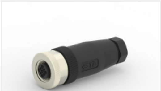
TE Part #T4110001041-000 M12,FEMALE,STRAIGHT,A CODE,4P,PG7,GOLD
