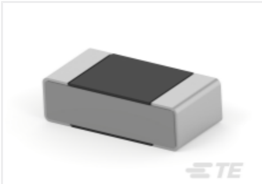
TE Part #1-2176280-1 CPF 0402 124K 0.1% 25PPM 1K RL
