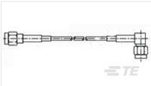
TE Part #1337811-2 50 OHM COAX SMA STR PLUG ELB P
