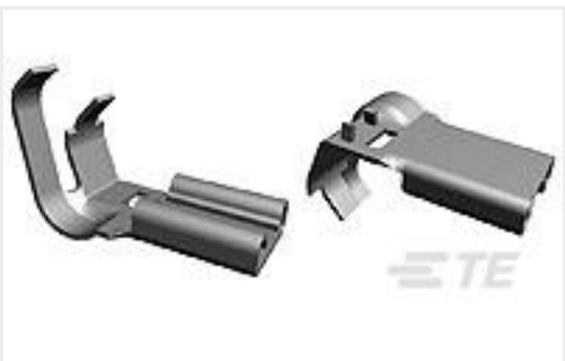
TE Part #180430-2 250 FASTON, FLAG, REC., 20-16 AWG, TPBR
