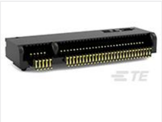
TE Part #1-2199119-6 M.2 0.5PITCH 3.2H KEY M 30U" AU
