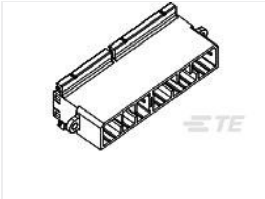
TE Part #1-174939-1 070 MLC CAP HSG 30P W/FLANGE
