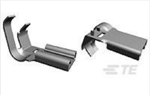
TE Part #180430-2 250 FASTON,FLAG,REC.,20-16 AWG, TPBR
