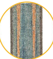
Example of damaged pin plating
