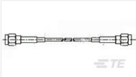
TE Part #1337808-2 50 OHM COAX SMA STR PLUG STR P
