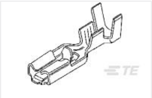
TE Part #63195-1 PL 187 RECEPTACLE 20-16 AWG TPBR
