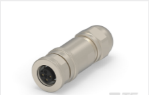
TE Part #T4110011031-000 M12 F, 3P GOLD A_CODE S SHIELDED PG7
