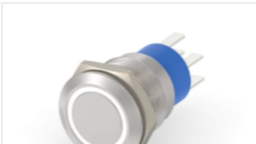
TE Part #6-2213767-3 AV19 DPL 3A MOVE RING LED WHITE 24V
