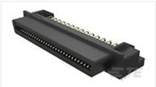
TE Part #1734037-5 Champ 050 series,50pos,Au over PdNi
