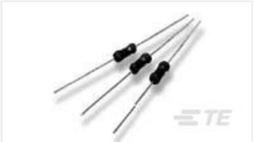
TE Part #7-1625890-0 2W SM M/OX 5% 82K
