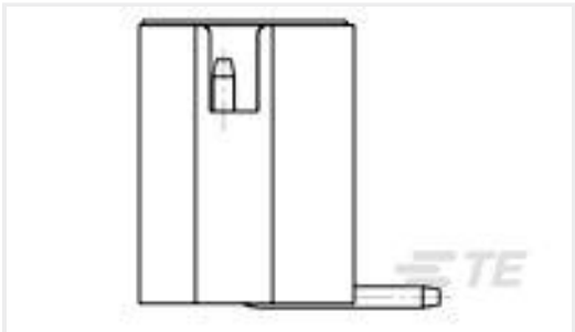
TE Part #1775470-2 HPI CONN., 2.0MM, V/T, SMT, 2P, 80U"
